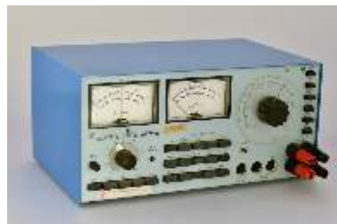
Figure 4.3: Bang & Olufsen WM1, analogue wow and flutter meter.
