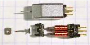
Figure 3.4: A disassembled MMC 1 cartridge. This magnetic circuit is slightly different than that shown in the diagram above. In this case, the magnet is the small square with the hole, shown on the right side of the photo. This is mounted at the front of the pickup instead of the rear. Note that the paper is ruled in 5 mm squares.
