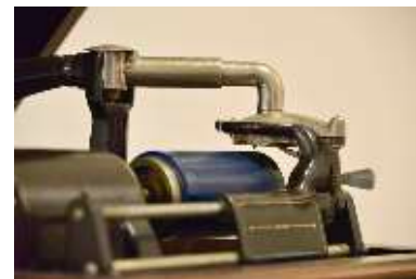
Figure 2.8: A closeup of the Edison player. Notice that the needle is mounted to move vertically, modulating a membrane located at the end of the tonearm (the bent pipe).
